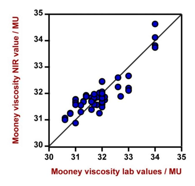
**Figure 3.** Correlation diagram and the respective figures of merit for the prediction of Mooney viscosity in BIIR using a DS2500 Liquid Analyzer. The lab values were evaluated using a Mooney viscometer.
