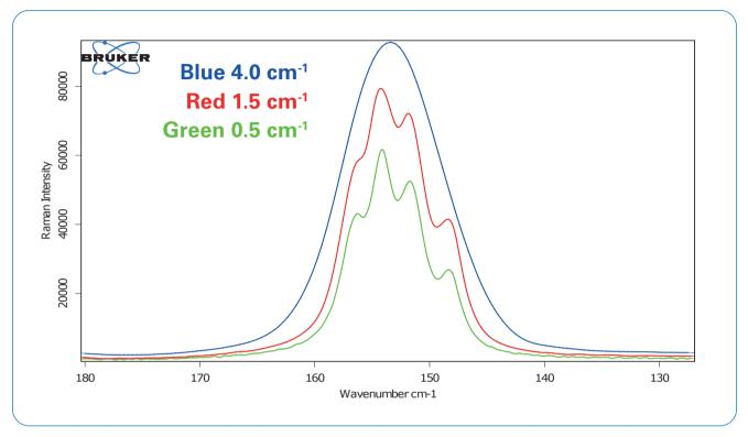
Figure 3: The Raman line of Sulfur at 153 cm<sup>-1</sup> acquired at different spectral resolutions with different instruments: Blue: 4.0 cm<sup>-1</sup> by SENTERRA II, 532 nm, grating: 400 gr/mm; Red: 1.5 cm<sup>-1</sup> by SENTERRA II, 532 nm, grating 1200 gr/mm; Green: 0.5 cm<sup>-1</sup> by MultiRam FT-Raman, 1064 nm.
