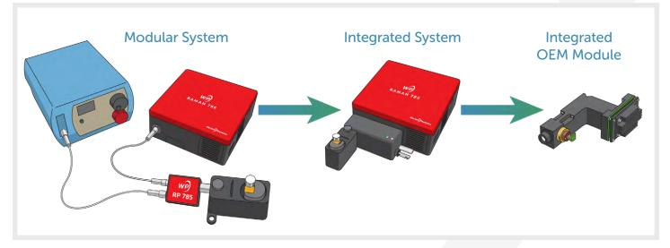
The advantage of this approach to product design is that proof of concept testing and initial research can be performed with modular components to keep the system as flexible and reconfigurable as possible, and with the confidence that important factors like sensitivity, thermal stability, and unit-to-unit variability have already been addressed in the core spectrometer design and will remain consistent throughout the integration process.
