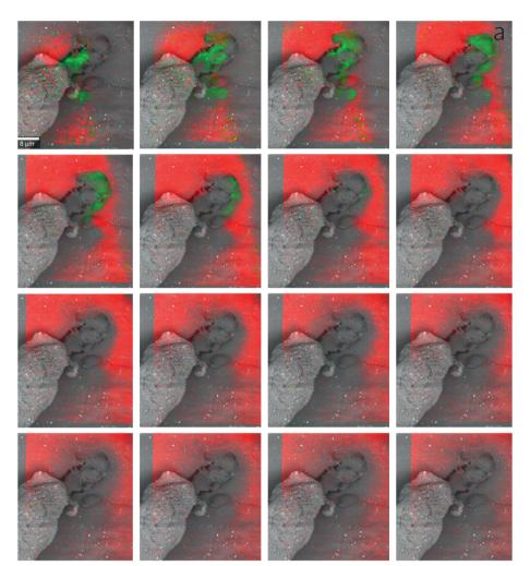
Fig 6: 3D imaging of SWCNTs on PE film. For a 3D image of the SWCNTs on PE sample 16 equidistant Raman images were taken while the focus was shifted by 1 µm for each image. The individual images are displayed as RISE images in (a). The compiled 3D Raman image of the analyzed sample area shows the SWCNTs located on the top of the PE filter (b). Image parameters: 200 x 200 µm<sup>2</sup> scan range, 70 x 70 pixels = 4,900 spectra, integration time: 0.037 s/
