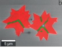
Fig. 7: (a) SEM image of MoS<sub>2</sub> twin crystals (b) Raman spectra of MoS<sub>2</sub> monolayers (red), two or more layers (green) and silicon (purple). (c) corresponding color-coded Raman image derived from the spectral information overlaid on the SEM image to give the RISE image. Image parameters: 22 x 17  $\mu$ m<sup>2</sup> scan range, 65 x 50 pixels = 3,250 spectra, integration time: 0.037 s/spectrum.
