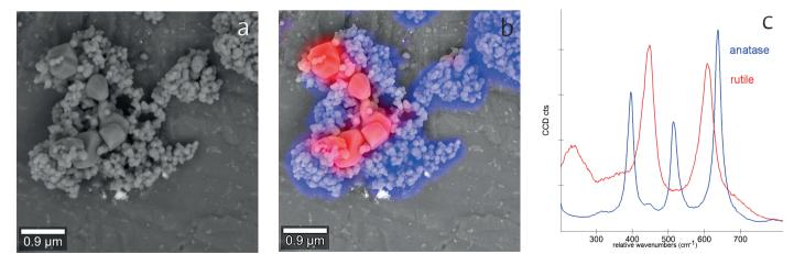
Figure 8: Two modifications of TiO2, anatase and rutile, were mixed 1.1, ground, dissolved in water and imaged with an SEM (a) and a confocal Raman microscope. (b) SEM and Raman images overlaid. (c) In the Raman spectrum anatase (blue) can be easily distinguished from rutile (red). Image parameters: 12 x 12 µm<sup>2</sup> scan range, 150 x 150 pixels = 22,500 spectra, integration time: 0.037 s/spectrum.
