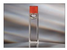
Figure 1. Sealed certified wavelength reference.
