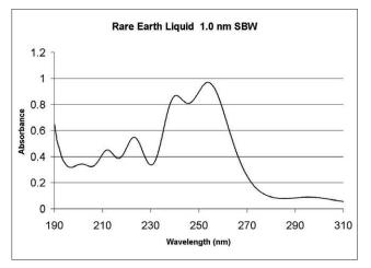
Figure 2. Wavelength scan of certified far-UV wavelength reference, recorded at 1nm spectral bandwidth.
