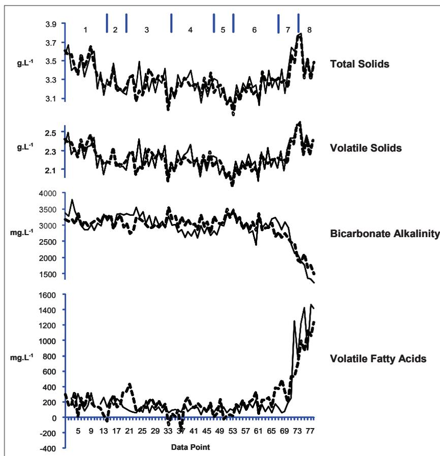
**Figure 6.** Application of the PLS model to tracking the reactor analyte concentrations in real time. This data is from reactor one, the solid line is the measured value and the dashed line the predicted value. The scale on the top of the figure indicates the different operating condition periods.
