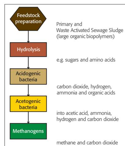
**Figure 2.** High-level flowchart showing the different stages of anaerobic digestion as well as the products and intermediates.
