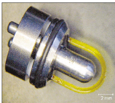
Figure 5. Exchangeable tips for silver halide IR fibre probes.
