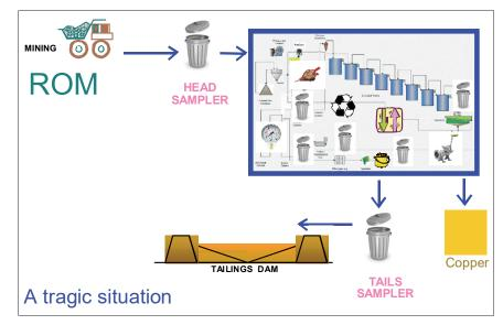
**Figure 2.** It is impossible to monitor and control a complicated process based only on seriously compromised sampling stations at input and output locations (here represented by the caricature of trash cans—perhaps a bit rude but this does allow the message to get through with clarity.
