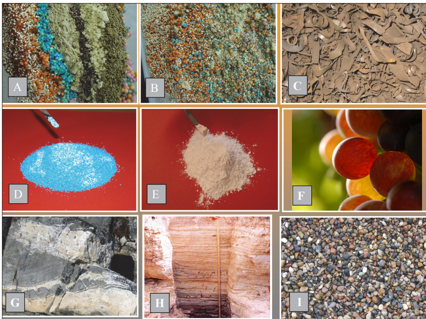
Figure 2. The phenomenon of heterogeneity is intrinsic to each lot material (always displaying both a compositional as well as a spatial component, CH and DH). For this understanding, which determines the necessary sampling process (composite sampling always—never grab sampling), it does not matter what came before. It is actually immaterial that of the “lots” depicted only panels F, G and H are primary lots—all other panels depict samples from a particular later stage in the generic “from-lot-to-aliquot” pathway.
