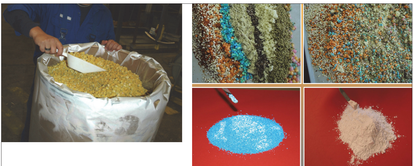
Figure 3. Mesoscale grab sampling (left) vs micro-scale in the lab. (right)—what is the difference? This is the wrong question, at the wrong time and at the wrong place (scale)—what matters is that heterogeneity follows suit all the way to the final aliquot extraction. It truly does not matter whether the human eye can discern any material heterogeneity, or not—60+ years of experience allows TOS to state categorically that all materials are significantly heterogeneous and shall therefore be treated accordingly. This insight actually makes all of sampling immensely easy: act as if all lots, all materials, at all scales are always heterogeneous.
