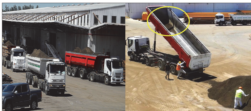
Figure 4. Left: Trucks moving in a port area from storage, via a weighbridge to quayside for discharge (v.v.). Right: Truck tipping cargo at quay for loading onto a receiving vessel. Inside the yellow circle 2000 kg of cargo remnants are visible that will remain inside the truck during its next trip (wIEE).
