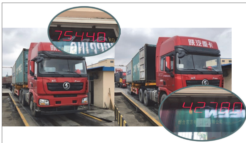
Figure 3. Full (container doors closed) container on truck: gross mass. After discharge, the empty container (doors open), the truck is weighed again: tare mass. The difference will be the cargo mass.
