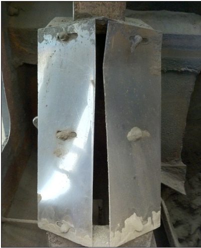
Figure 1. Falling stream cutter with contorted edges that result in incorrect delineation (IDE).
