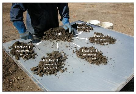
**Figure 2.** Primary samples obtained from the piles shown in Figure 1, which were reduced in the field using fractional shovelling as shown. Each fraction correspond to a final field sample sent to the laboratory. Secondary sample mass thus obtained was approximately 600 g of dry matter.
