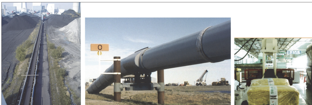
Figure 1. Dynamic (moving) 1-dimensional lots, from left to right: a conveyor belt transporting coal to a power plant, a pipeline, a series of produced goods). Photo credit: Hans Møller, with permission, and KHE.
