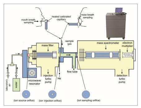
**Figure 1.** Schematic of the current Profile 3 SIFT-MS instrument and a photograph (the laptop gives the scale). Also illustrated are both mouth and nose-exhaled breath sampling.
