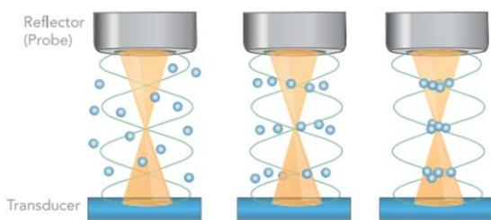
Figure 8: An ultrasonic standing wave formed between a piezo transducer and a Raman probe used as the reflector captures small particles in the nodes
