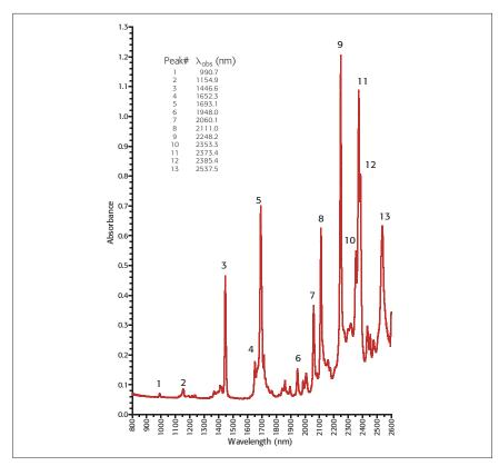
Figure 2. NIR absorbance spectrum of TS5 800–2600 nm on a Cary 500 spectrometer 0.5 nm SBW and 0.05 nm data pitch.<sup>10</sup>
