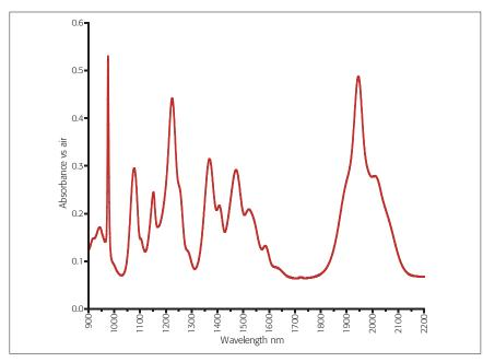
Figure 1. SRM 2035 FT-NIR spectrum at 8 cm<sup>-1</sup> resolution.<sup>9</sup>
