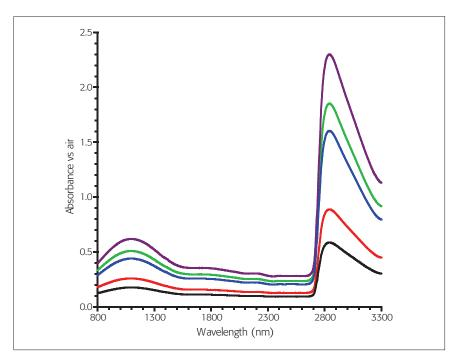
Figure 3. Typical Schott NG glass spectra in the NIR.
