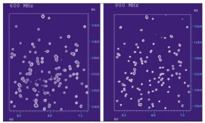
Figure 2. 2D N–H correlated TROSY spectra of a 1 mMol protein (sample courtesy of Dr L. Mueller) in  $H_2O/D_2O$  (9 : 1) recorded at 600 MHz and 900 MHz on a Varian INOVA spectrometer (courtesy of Varian).
