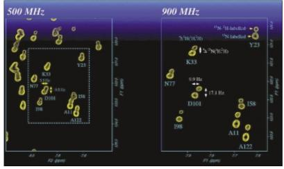
Figure 3. N–H correlated TROSY spectra of a mixture of H- and D-Lysozyme (sample courtesy of Dr C. Redfield) in  $H_2O/D_2O$  (9:1) recorded at 500 MHz and 900 MHz on a Varian INOVA spectrometer (courtesy of Varian).
