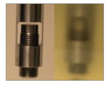
**Figure 1.** Transflectance probe used for data collection. Left panel shows the design of the probe with the adjustable pathlength. Right panel shows probe inserted into cell culture during data collection.
