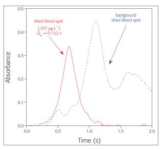
**Figure 3.** Signal profile obtained for Pb from dried blood spot using the temperature programme detailed in Table 1.
