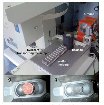
**Figure 2.** Different steps for Pb determination in blood from dried blood spots by FP-SS-GFAAS. (1) Solid Sampling device including a sample tray, a pair of tweezers and a microbalance. The tweezers are transporting the sample towards the furnace. (2) Detail of the platform containing the blood spot together with the modifier solution. (3) Carbonaceous residue left after carrying out the temperature programme.
