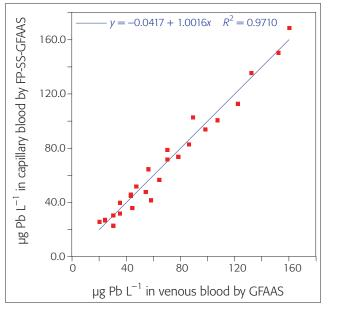
**Figure 4.** Linear least squares regression analysis of blood lead contents obtained for paired samples from 25 patients using two methodologies: FP-SS-GFAAS (y-axis) vs analysis of venous samples by solution GFAAS (x-axis).
