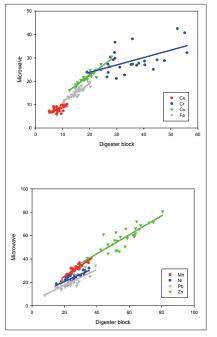
Figure 1. Comparison of heavy metal concentrations (mgkg<sup>-1</sup>) obtained in the Lower Segura basin (n=29) by digester block and microwave oven. Fe concentrations have been divided by 1000 and Mn concentrations have been divided by 10.
