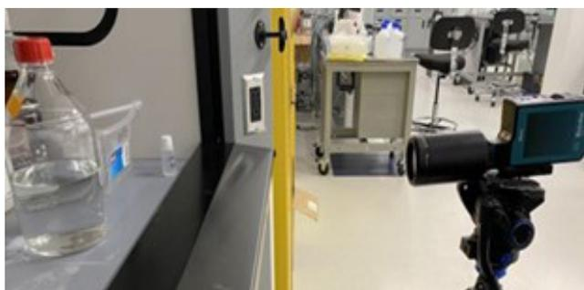
**Figure 4.** Setup of identifying polyphenyl isocyanate through sealed glass container at 0.5 meters using the manual standoff.
