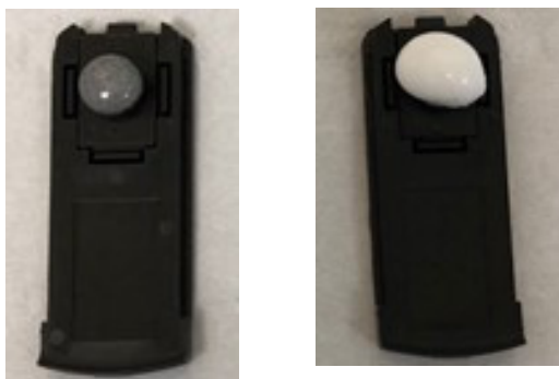
Figure 3: Images showing the lamination adhesives before (left) and after (right) curing
