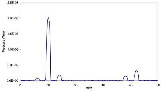
Figure 1: Profile scan for 10000ppm NO<sub>2</sub>.
