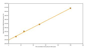
Figure 3: Relationship between partial pressure for m/z 30 and NO concentration (Note: The background at m/z 30 due to  $NO_2$  has been subtracted).
