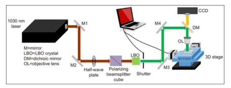
Figure 1. Schematic of laser fabrication system for microfluidic SERS chips. Credit: OEA
