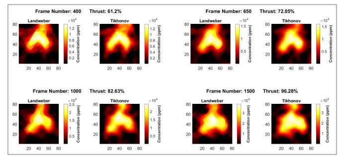
The researchers used their new chemical species tomography setup to capture the first images of carbon dioxide exhaust from a commercial aircraft engine. At all thrust levels, a ring-structure of high carbon dioxide concentration can be seen in the central region of the engine. Credit: Abhishek Upadhyay, University of Strathclyde
