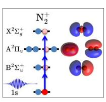
Watching the fate of molecular nitrogen with X-rays, when an electron has been kicked out. Copyright: MBI /E.T.J. Nibbering / C. Kleine
