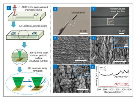
**Figure 2.** (a) Schematic of the fabrication; (b) photograph of microfluidic SERS chip; (c) optical microscope image showing the SERS substrate. SEM images of (d) original metal film, (e) ripples generated by first laser scanning and (f) nanodots generated by second laser scanning (insert: low magnification of SEM image). (g) Raman spectra of  $10^{-9}$  M Rhodamine 6G (R6G) on 2-D (black) and 1-D (red) nanostructured SERS substrates. Credit: OEA
