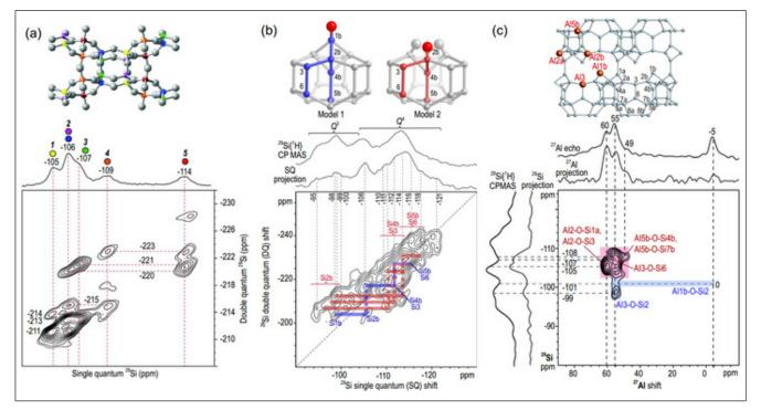
(a) 2D refocused INADEQUATE (J-mediated) <sup>29</sup>Si{29Si} DQ NMR spectrum of as-synthesised zeolite ITW. (b) DNP-enhanced 2D <sup>29</sup>Si{29Si} J-mediated correlation spectrum of calcined Si-SSZ-70. (c) Schematic diagram of the framework structure of Al-SSZ-70 (orange indicates the T sites that are occupied by Al heteroatoms), and 2D <sup>27</sup>Al{29Si} J-HMQC NMR spectrum of calcined Al-SSZ-70. Credit: ©Science China Press
