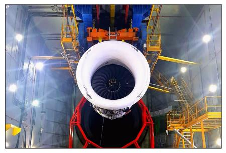
Researchers developed a technique called chemical species tomography that can capture carbon dioxide exhaust from a commercial airplane engine. To image such a large area, the researchers used a 7-m diameter optical mounting frame (red) located just 3 m from the exit nozzle of the engine. The testing facility is at the Instituto Nacional de Tecnica Aeroespacial (INTA) in Madrid. Credit: Gordon Humphries, University of Strathclyde
