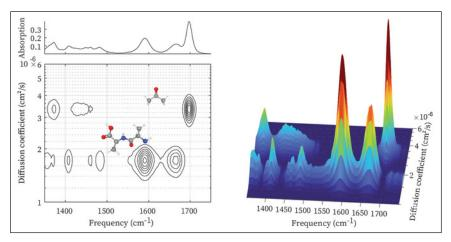
IR-DOSY spectra of a mixture of acetone and dialanine, showing which IR peak belongs to which compound. Credit: HIMS
