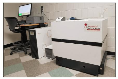
**Figure 1.** A Varian EM360 which has been upgraded through the Anasazi Instruments "Refresh Program" (<u>https://www.aiinmr.com/EM-360-NMR-Refresh-</u> Program). Image courtesy Anasazi Instruments
