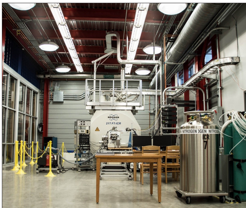
Researchers are using a 21 T FT-ICR mass spectrometer to identify and analyse “forever” chemicals. Credit: National Maglab
