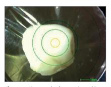
**Figure 1.** Photograph of contaminant (the yellow circle is the x-ray irradiation range:  $1 \text{ mm } \mathcal{D}$ ).
