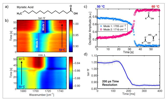
**Figure 2.** Time-resolved IR laser ellipsometry of the solid-to-liquid phase transition of a fatty-acid thin film upon heating/cooling. a) Chemical structure of MyA. b)  $\nu$ (C=O) band amplitude and phase during slow heating. c) Oscillator amplitudes of mode 1 and 2 fitted from the spectral images. Reprinted with permission from Reference 13 (©2019, Optical Society of America). d) Sub-ms single-wavelength monitoring of mode 1 during rapid cooling.
