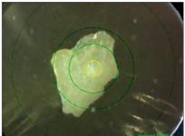
**Figure 4.** Photograph of contaminant (the yellow circle is the x-ray irradiation range: 1 mm  $\emptyset$ ).
