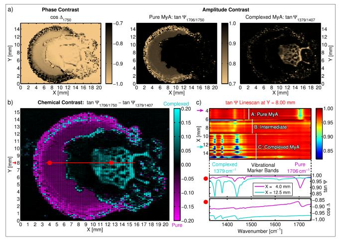
**Figure 1.** Hyperspectral IR ellipsometry images of a partially chemically modified, drop-cast MyA film. a) Phase and amplitude contrast at different wavelengths. b) Chemical contrast between pure and complexed MyA. c)  $\tan \Psi$  linescan across the heterogeneous sample surface and exemplary ellipsometric spectra. Reprinted with permission from Reference 8 (©2019, Optical Society of America).
