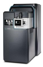
every pass, greater ion mobility resolution is achieved. The cyclic device provides scalable, high-resolution ion mobility separations and introduces the unique ability to perform ion mobility/ion mobility and IMS<sup>n</sup> experiments, extending the benefits of routine ion mobility.
