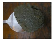
**Figure 3.** Mercury flour (droplets) in a spoonful of tailings (Philippines). Reproduced from Reference 7 with permission.
