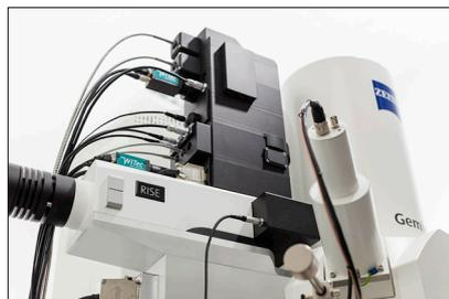
WITec's RISE system for correlative Raman/SEM imaging is now available on the Zeiss Sigma 300.
