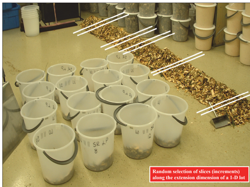
Figure 2. There should always be an element of randomness in a good sampling procedure, here the locations along the extension dimension of a 1-D lot are selected in this fashion. All slices correspond to complete slices of the width–height dimensions of the lot. Illustration credit: KHE.
