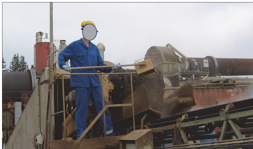
Figure 6. Manual increment extraction from a conveyor belt defining a dynamic 1-D lot. The scoop used to extract increments is less than half the width of the conveyor belt, imparting significant incorrect sampling error effects to the process sampling. This results in an (unnecessarily) inflated nugget effect, which is one of the means by which variographic process characterisation can also be used for total sampling-plus-analysis system evaluation, see, e.g., References 1 and 3. Photo credit: KHE
