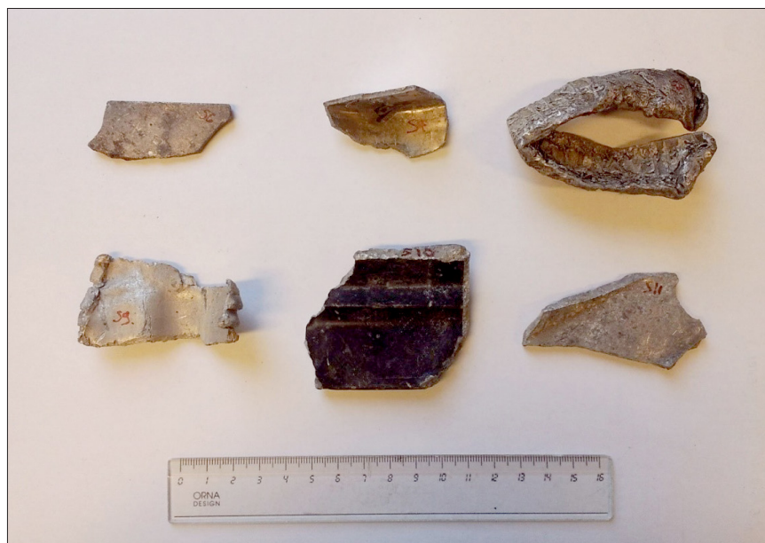
Figure 4. Some aluminium scraps used for laboratory tests in the SHREDDERSORT project.
