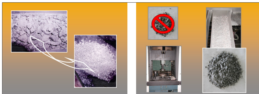
Figure 7. More efficient crushing leads to a much more uniform material in the loading tray, especially when combined with a conscious effort for better mixing as well.
