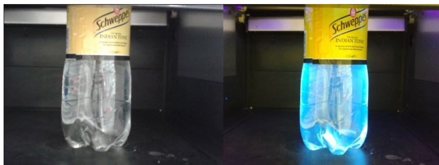
Figure 1. Tonic water illuminated with visible light (left) and a UV lamp (right). The glowing blue colour is due to the fluorescence of quinine.
