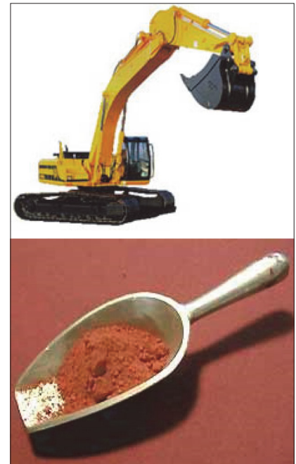
Figure 4. Sampling tool size is set to match the lot size first, but the key function of any sampling tool is always to counteract the material heterogeneity present (CH, DH); see also Figure 3.
