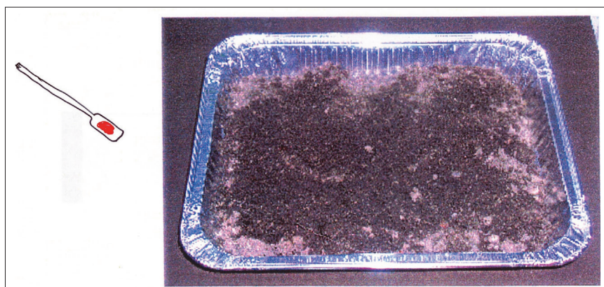
Figure 1. The laboratory—the realm of the spatula. At this ultimate stage of the long sampling pathway from the original lot, significant sampling errors can still crop up, mostly due to a faulty understanding that if the material appears homogenous this justifies grab sampling, spatula sampling. NOTHING could be further from the truth, however.
