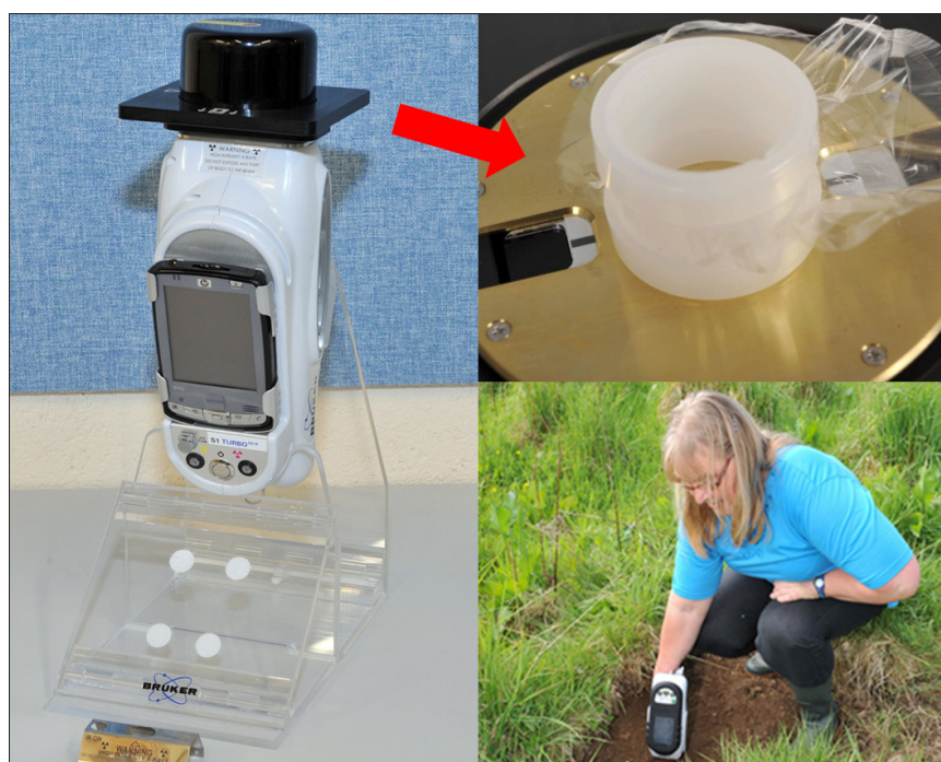
Figure 2. Portable XRF instrument on stand with sample holder and film located under the radiation shield. The inset (bottom right) shows portable XRF being used in the field.
