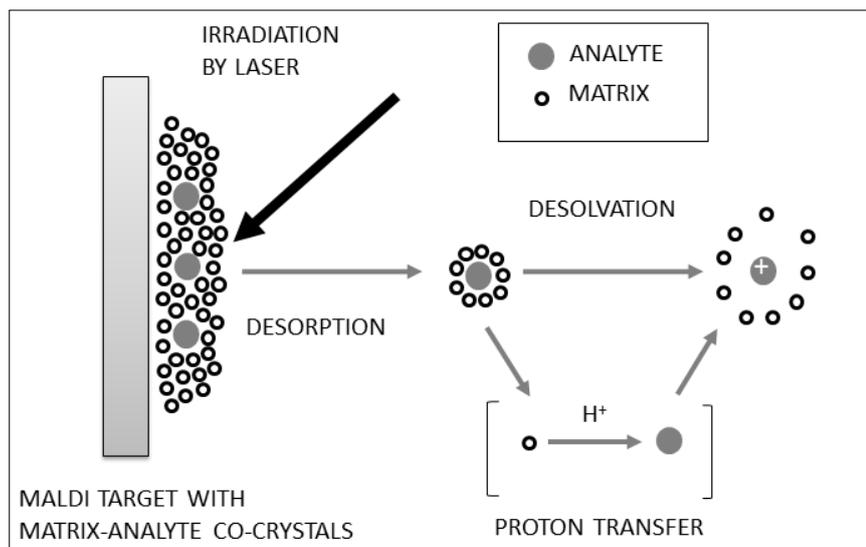
**Figure 1.** A scheme of the principle of MALDI (adapted from a previous publication<sup>7</sup>).
