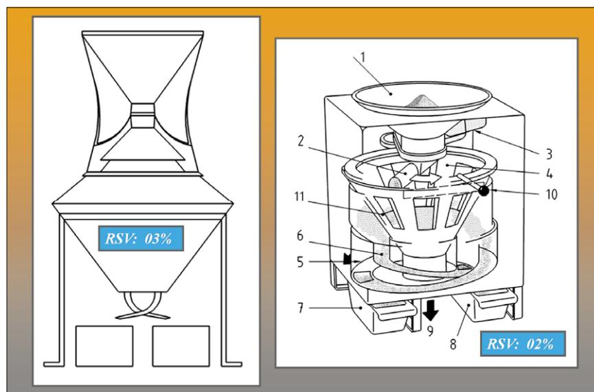
**Figure 6.** Two laboratory equipment (splitters) subjected to RE assessment, showing highly satisfactory quantitative results. N.B. illustrative examples only, no specific sampler is endorsed, nor renounced. Samplers are sketched only in order to illustrate how RE may be used for quantitative assessment.
