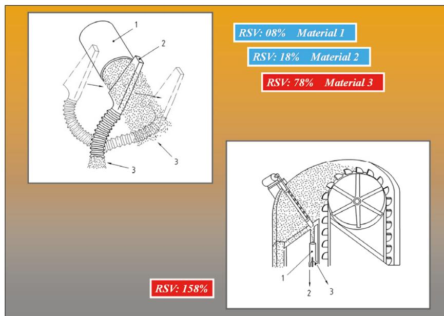
**Figure 5.** Upper left: primary process sampler assessed for three different materials, one of which does not pass the test of the dedicated RE ( $RSV=78\%$ ). Lower right: a complex primary sampler being subjected to a RE with the distinctly worrisome result of  $RSV=158\%$ . N.B. illustrative examples only, no specific sampler is endorsed, nor renounced. Samplers are sketched only in order to illustrate how RE may be used for quantitative assessment.
