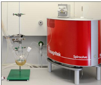
Magritek have released new solutions that enable reaction monitoring on the Spinsolve benchtop NMR spectrometer.
