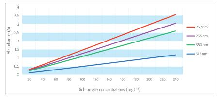
Figure 3. Potassium dichromate linearity.
