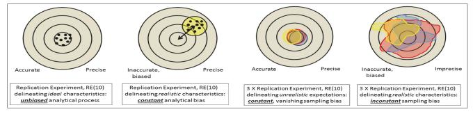
Figure 6. Analytical bias (left) vs sampling bias (right). Bias effects are shown as manifested by Replication Experiments (RE).
