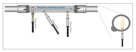
**Figure 2.** The "PAT sensor application solves all sampling issues" fallacy, which follows because PAT sensors are not "seeing" a volume corresponding to a full cross-sectional **slice** of a moving stream of matter, see also Figure 3. Illustration copyright KHE Consulting and Martin Lischka, reproduced with permission.
