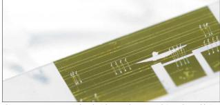
Chip spectrometer, ~2cm in length. (Photograph: ETH Zurich/Pascal A. Halder)
