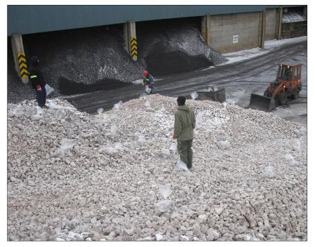
**Figure 1.** Overview of the experimental design (note plastic bags each containing 10 kg, see text). Student and supervisors hard at work on a typical industrial lot of raw material, quartzite. Note that all inspection and sampling takes place on the lot surface, following years of experience with the overall heterogeneity of truckload lots transported from the mine. Photo courtesy of Dany Desroches.
