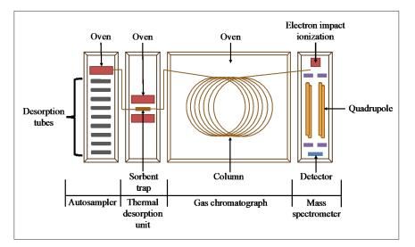
**Figure 1.** Illustration of various steps of thermal desorption hyphenated to gas chromatography/ mass spectrometry, adapted and modified from Materic *et al.*<sup>7</sup>
